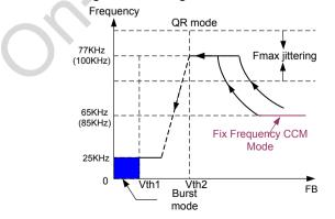
At full load conditions, there are two situations: firstly, if the system input is in low line input range, the IC operates in 85K fixed frequency CCM mode. Thus, small size transformer can be used with high power conversion efficiency. Secondly, if the system input is in high line input range, the IC operates in QR mode. In this way, high power conversion efficiency can be achieved in the universal input range when system is at full loading conditions.
