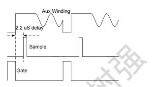
The auxiliary winding voltage is a well-defined replica of the output voltage. The OTP works by sampling the plateau voltage at CS pin during the flyback phase. OB2710 can sample this flat voltage level after a delay time to perform over temperature protection. This delay time is used to ignore the voltage ringing from leakage inductance of PWM transformer.
