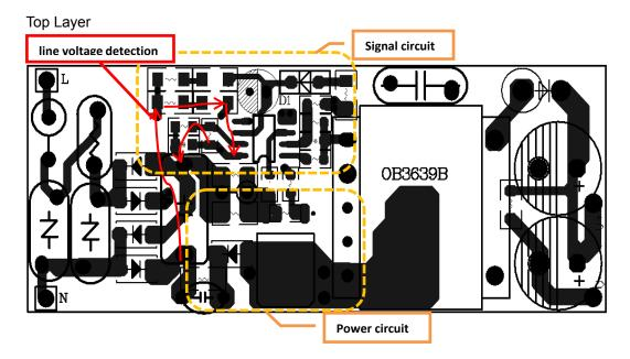
2) Power circuit area as small as possible, reduce high frequency noise. It is shown below:
