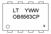
Y:Year Code(0-9) WW:Week Code(01-52) C:SOP8 Package P:Pb-free Package S:Internal Code(Optional)
