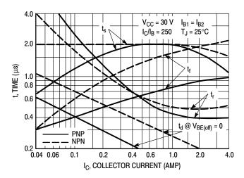
Figure 2. Switching Times
