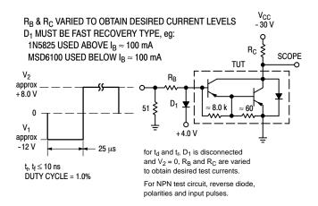
Figure 1. Switching Times Test Circuit
