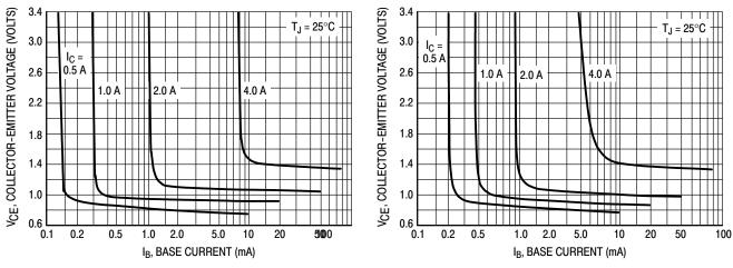
Figure 8. Collector Saturation Region
