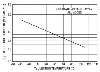
Figure 6. Typical Gate-Trigger Current
