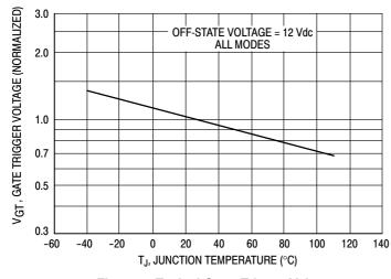
Figure 5. Typical Gate-Trigger Voltage
