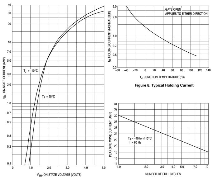
Figure 7. Maximum On-State Characteristics
