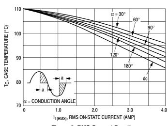
Figure 2. RMS Current Derating
