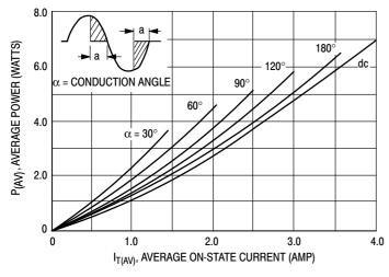
Figure 3. Power Dissipation
