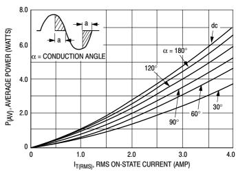
Figure 4. Power Dissipation
