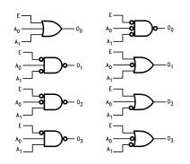
Figure 1. Gate Functions (Each Half)
