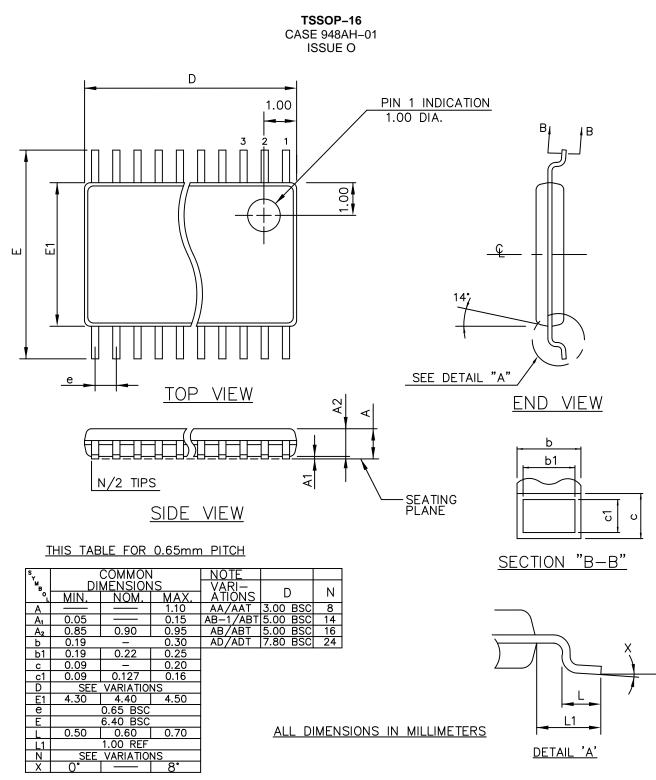
MOLD FLASH OR PROTRUSIONS SHALL NOT EXCEED 0.15mm ON D PER SIDE
