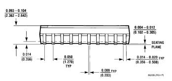
Figure 1. 20-Lead Small Outline Integrated Circuit (SOIC), JEDEC MS-013, 0.300" Wide Package Number M20B
