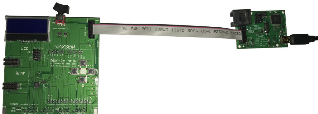
Figure 3. DVK-2 Main Board Connected to the AXDBG
