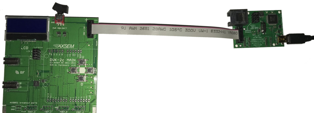
Figure 3. DVK-2 Main Board Connected to the AXDBG
