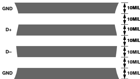
Figure 34. Arrangement of Signal Tracks
