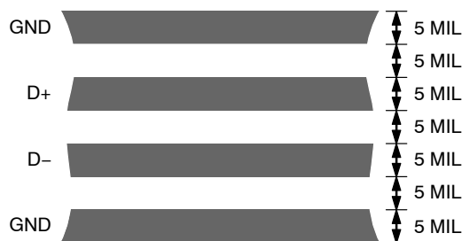
Figure 22. Typical Arrangement of Signal Tracks
