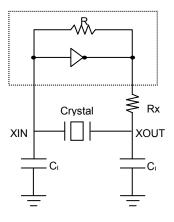
$C_L$  = 2\*(C\_P - C\_S), Where  $C_P$  = Load capacitance of crystal from crystal vendor datasheet.  $C_{S}$  = Stray capacitance due to  $C_{IN}$ , PCB, Trace, etc.
