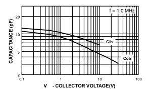
Figure 7. Input and Output Capacitance vs. Reverser Voltage
