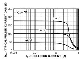
Figure 1. Typical Pulsed Current Gain vs.
