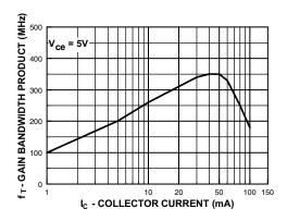
Figure 8. Gain Bandwidth Product vs. Collector Current
