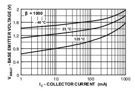
Figure 3. Base-Emitter Saturation Voltage vs.
