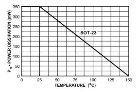
Figure 9. Power Dissipation vs. Ambient Temperature
