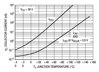
Figure 18. Typical Collector Leakage Current
