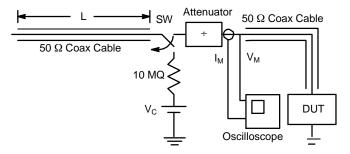
Figure 5. Simplified Schematic of a Typical TLP System
