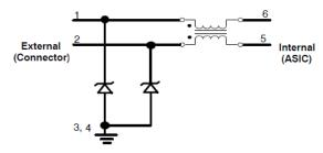
Figure 1. EMI8131 Electrical Schematic
