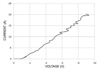
Figure 5. Negative TLP I-V Curve
