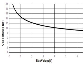
Figure 3. Filter Capacitance vs. Input Voltage (Normalized to Capacitance at 0 VDC and 25°C)
