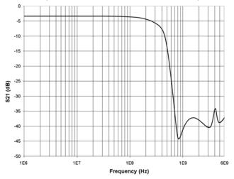
Figure 2. Typical Filter Insertion Loss
