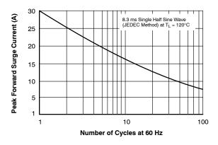
Figure 2. Maximum Non-repetitive Peak Forward Surge Current
