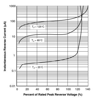
Figure 4. Typical Reverse Characteristics
