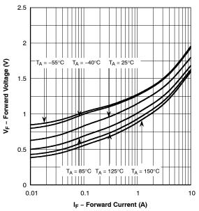
Figure 3. Forward Current vs. Forward Voltage
