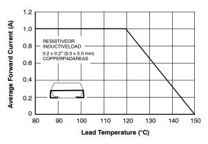
Figure 1. Maximum Forward Current Derating Curve
