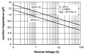
Figure 5. Typical Junction Capacitance
