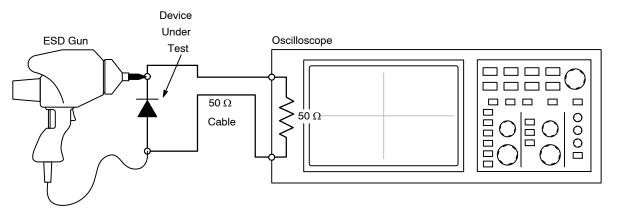
Figure 10. Diagram of ESD Test Setup
