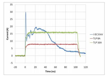
Figure 10. Comparison Between 8 kV IEC 61000-4-2 and 8 A and 16 A TLP Waveforms
