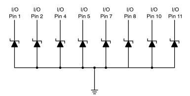
Center Pins, Pin 3, 6, 9, 12, 13, 14 Note: Common GND – Only Minimum of 1 GND connection required
