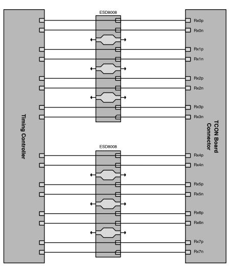
Figure 15. V-by-One HS Layout Diagram (for LCD Panel)
