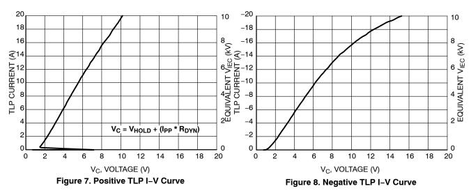
NOTE: TLP parameter:  $Z_0 = 50 \Omega$ ,  $t_p = 100$  ns,  $t_r = 300$  ps, averaging window:  $t_1 = 30$  ns to  $t_2 = 60$  ns.  $V_{IEC}$  is the equivalent voltage stress level calculated at the secondary peak of the IEC 61000–4–2 waveform at t = 30 ns with 2 A/kV. See TLP description below for more information.
