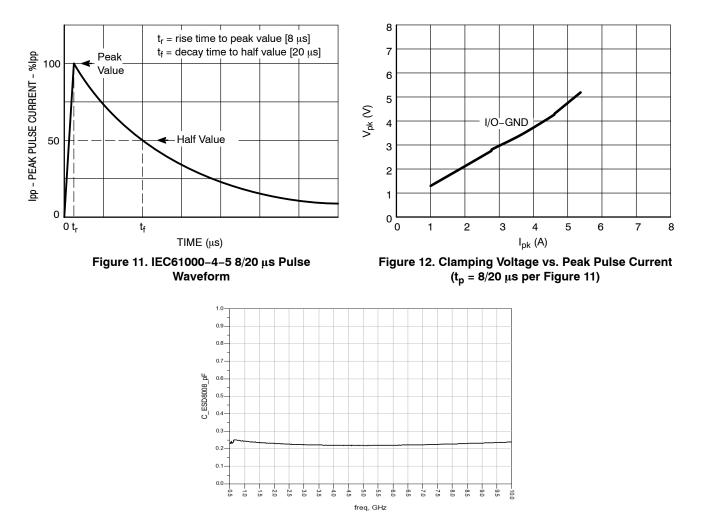
Figure 13. Junction Capacitance;  $V_R = 0$ , f = 500 MHz – 10 GHz
