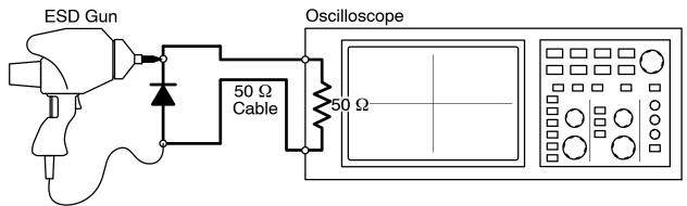
Figure 5. Diagram of ESD Clamping Voltage Test Setup
