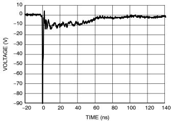
Figure 3. IEC61000-4-2 -8 kV Contact Clamping Voltage
