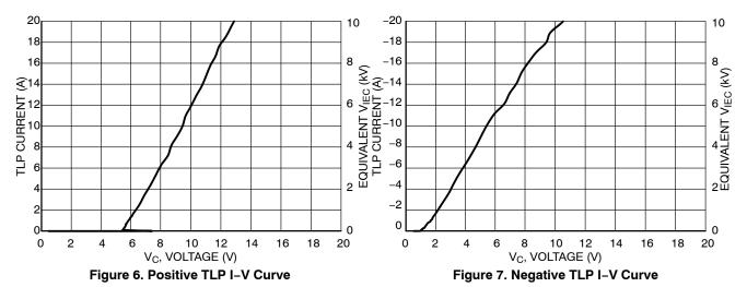
NOTE: TLP parameter: Z<sub>0</sub> = 50  $\Omega$ , t<sub>p</sub> = 100 ns, t<sub>r</sub> = 300 ps, averaging window: t<sub>1</sub> = 30 ns to t<sub>2</sub> = 60 ns. V<sub>IEC</sub> is the equivalent voltage stress level calculated at the secondary peak of the IEC 61000–4–2 waveform at t = 30 ns with 2 A/kV. See TLP description below for more information.
