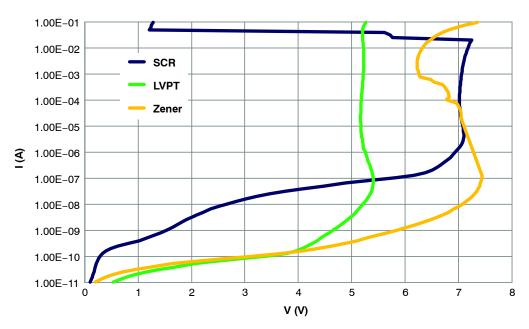
Figure 17. Low Current, DC, IV Characteristic of Each Technology
