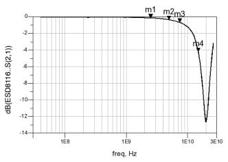
Figure 12. RF Insertion Loss
