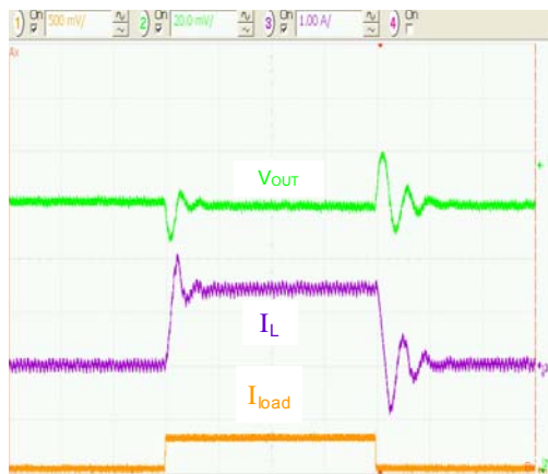
Figure 15. MODE=1, 100 mA to 1.5 A to 100 mA, 5 \mu\text{s}/\text{div} .
