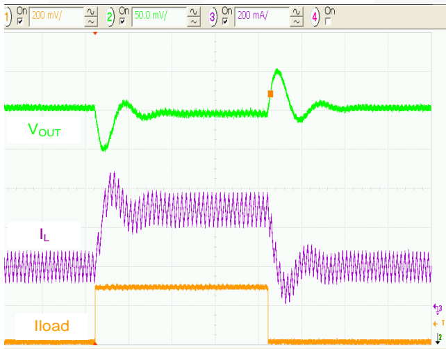
Figure 15. Load Transient 200 to 500mA, 3.6V IN , 5μs/div.
