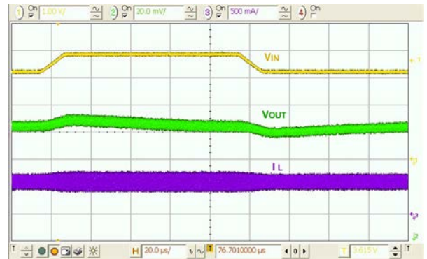
Figure 21. Line Transient, 3.3-3.9-3.3 V_{IN} , 10 \mu\text{s} Edge, 600 mA Load
