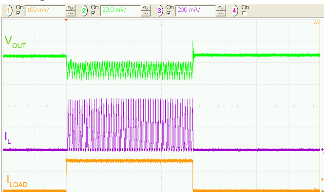
Figure 30. Load Transient 0 to 150 mA, 4.5 V_{IN}
