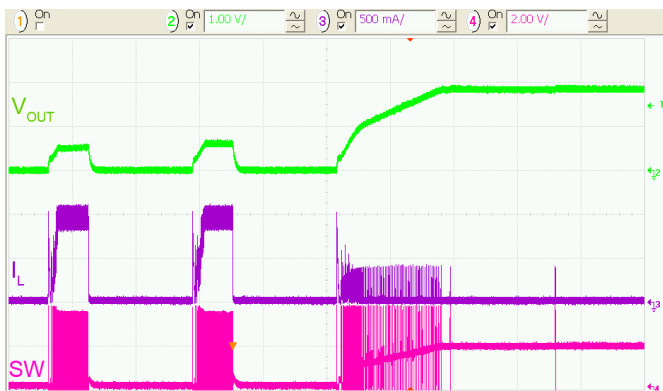
Figure 37. Overload Recovery to Light Load, 50\ \mu\text{s}/\text{div} .
