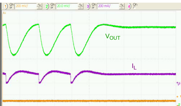
Figure 15. Regular Switching to 100% Duty Cycle Transition at V_{IN} = 3.2\text{ V} , 5\text{ }\mu\text{s/div}
