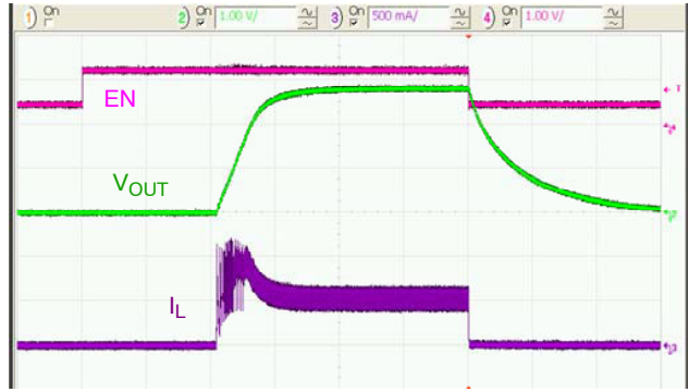
Figure 18. Startup and Shutdown through V_{EN} with 500 mA Load, 50 \mu\text{s} /div.
