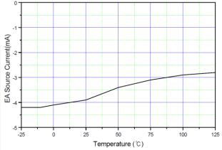
Figure 9. Startup Supply Current vs. Temperature
