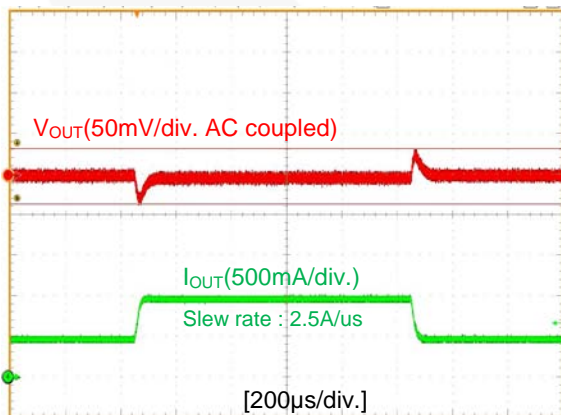
Figure 8. Load Transient Response(Step-up/down)
