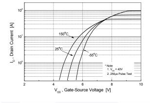
Figure 2. Transfer Characteristics
