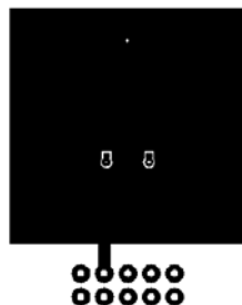
a) 40\text{ }^\circ\text{C}/\text{W} when mounted on a 1 in 2 pad of 2 oz copper
