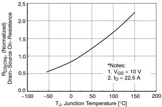
Figure 8. On-Resistance Variation vs. Temperature
