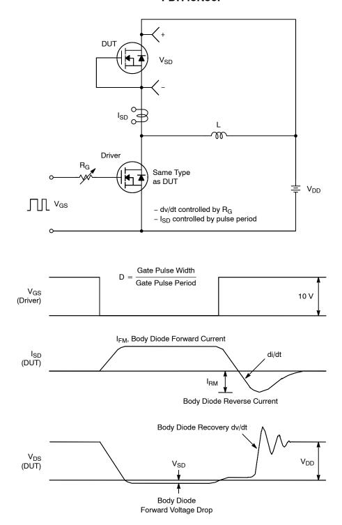
Figure 19. Peak Diode Recovery dv/dt Test Circuit & Waveforms
