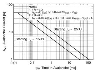
Figure 14. Unclamped Inductive Switching Capability
