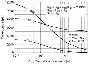
Figure 5. Capacitance Characteristics
