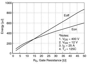
Figure 13. Typical Switching Losses vs. Gate Resistance
