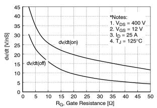
Figure 12. Typical Drain-Source Voltage Slope vs. Gate Resistance
