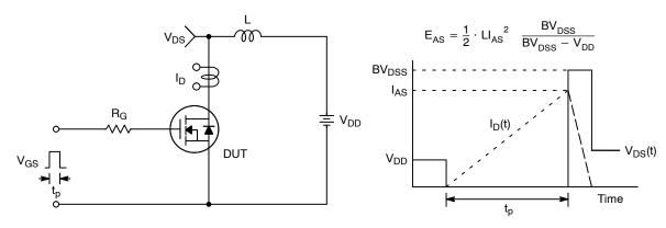
Figure 18. Unclamped Inductive Switching Test Circuit & Waveforms
