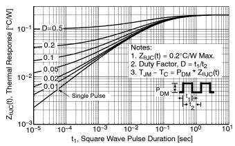
Figure 15. Transient Thermal Resistance Curve
