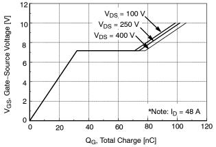
Figure 6. Gate Charge Characteristics
