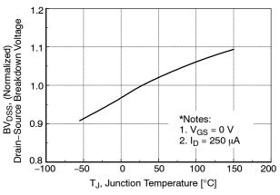
Figure 7. Breakdown Voltage Variation vs. Temperature
