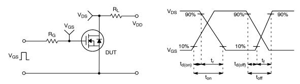
Figure 17. Resistive Switching Test Circuit & Waveforms
