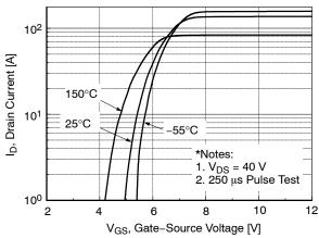
Figure 2. Transfer Characteristics
