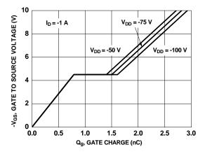
Figure 7. Gate Charge Characteristics
