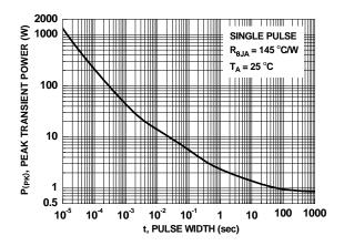
Figure 11. Single Pulse Maximum Power Dissipation
