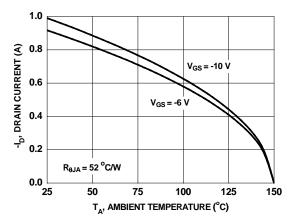
Figure 9. Maximum Continuous Drain Current vs Ambient Temperature
