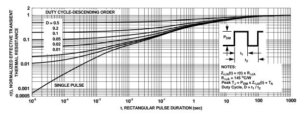
Figure 12. Junction-to-Ambient Transient Thermal Response Curve
