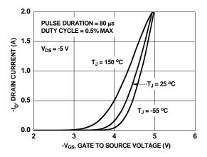
Figure 5. Transfer Characteristics
