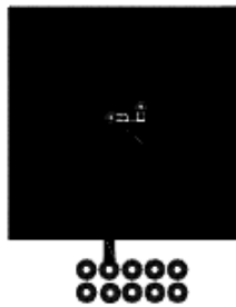
a. 65\text{ }^\circ\text{C/W} when mounted on a 1\text{ in}^2 pad of 2 oz copper.
