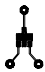
a. 250^\circ\text{C/W} when mounted on a 0.02\text{ in}^2 pad of 2oz Cu.
