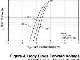
Figure 2. Transfer Characteristics
