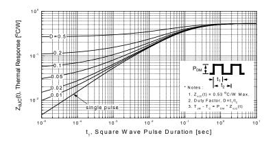
Figure 11-2. Transient Thermal Response Curve - FDPF18N50 / FDPF18N50T
