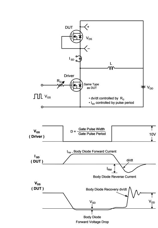
Figure 15. Peak Diode Recovery dv/dt Test Circuit & Waveforms
