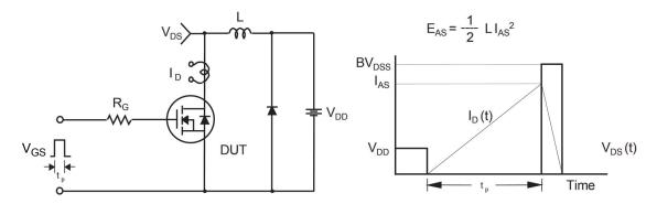
Figure 14. Unclamped Inductive Switching Test Circuit & Waveforms
