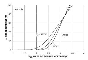
Figure 5. Transfer Characteristics.
