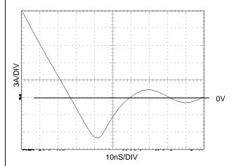
Figure 13. Non-SyncFET (FDS6690A) body diode reverse recovery characteristic.
