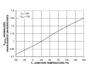
Figure 3. On-Resistance Variation with Temperature.
