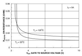
Figure 4. On-Resistance Variation with Gate-to-Source Voltage.
