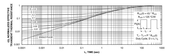
Figure 11. Transient Thermal Response Curve.
