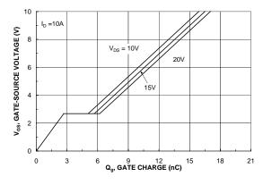
Figure 7. Gate Charge Characteristics.
