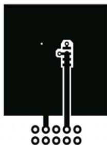
a.) 50°C/W when mounted on a 1 in 2 pad of 2 oz copper
