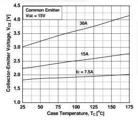
**Figure 2. Typical Output Characteristics**
