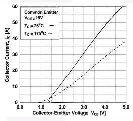
Figure 5. Saturation Voltage vs. Case
