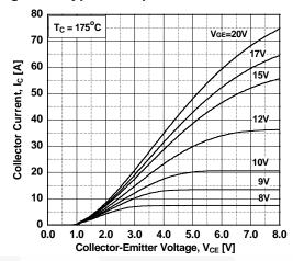
**Figure 4. Transfer Characteristics**
