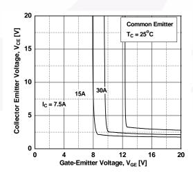
Figure 7. Saturation Voltage vs. V<sub>GE</sub>
