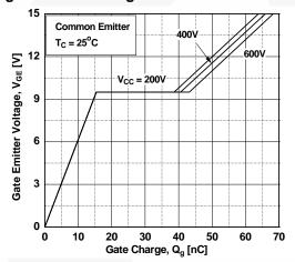
Figure 11. Turn-on Characteristics vs.
