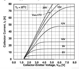
Figure 3. Typical Saturation Voltage Characteristics
