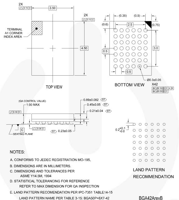
Figure 11. 42-Ball, Ball Grid Array (BGA) Package
