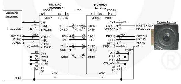
Figure 5. 8-Bit YUV 1.3MPixel CMOS Imager (Example Shows BGA 42-Pin Package)
