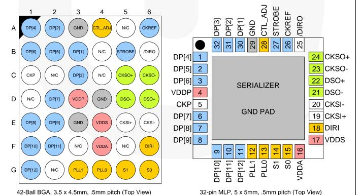
Figure 2. FIN212AC (Serializer DIRI=1) Pin Assignments (Top View)
