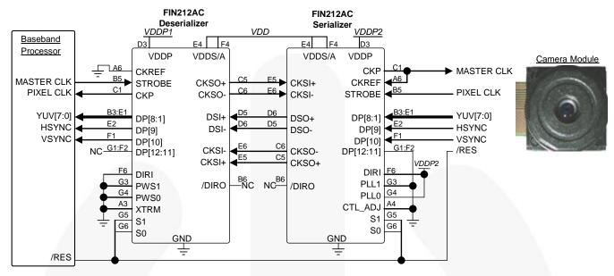
Figure 6. 8-Bit YUV 1.3MPixel CMOS Imager In Clock Pass-Through Mode
