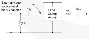
Figure 12. Biased SCART with AC-Coupled Outputs
