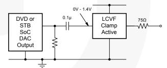
Figure 7. AC-Coupled Inputs, DC-Coupled Outputs
