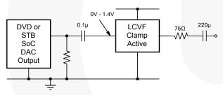
Figure 11. AC-Coupled Inputs and Outputs
