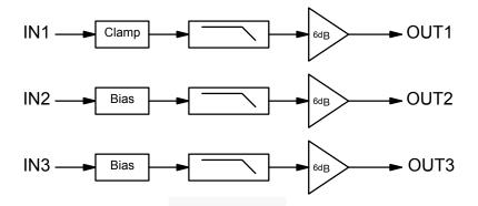
Figure 1. 7<sup>th</sup>-Order 30MHz Filter
