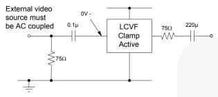
Figure 9. Biased SCART with DC-Coupled Outputs
