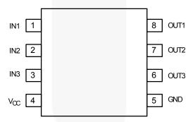
Figure 2. Pin Configuration
