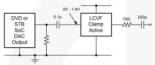
Figure 10. DC-Coupled Inputs, AC-Coupled Outputs
