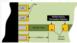
Figure 13. Termination Resistor
