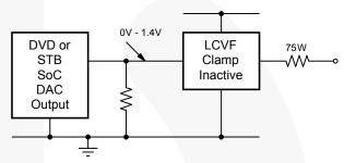
Figure 6. DC-Coupled Inputs and Outputs
