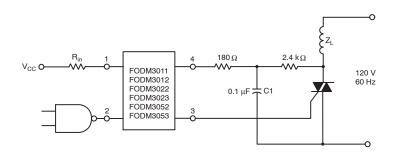
Figure 9. Inductive Load with Sensitive Gate Triac (IGT ≤ 15 mA)
