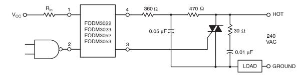
In this circuit the "hot" side of the line is switched and the load connected to the cold or ground side. The 39  $\Omega$  resistor and 0.01  $\mu$ F capacitor are for snubbing of the trisc, and the 470  $\Omega$  resistor and 0.05  $\mu$ F capacitor are for snubbing the coupler. These components may or may not be necessary depending upon the particular and load used.
