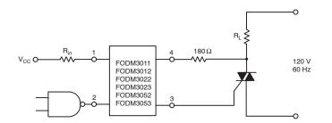
Figure 8. Resistive Load
