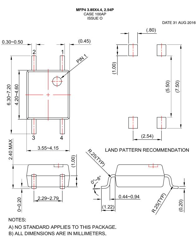
C) DIMENSIONS ARE EXCLUSIVE OF BURRS, MOLD FLASH, AND TIE BAR EXTRUSION
