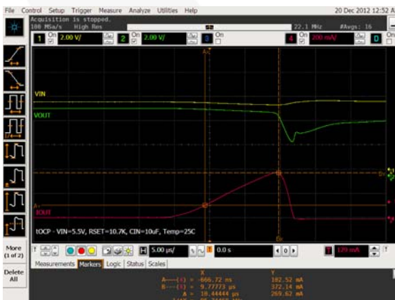
Figure 10. t_{OCP} Response Time
