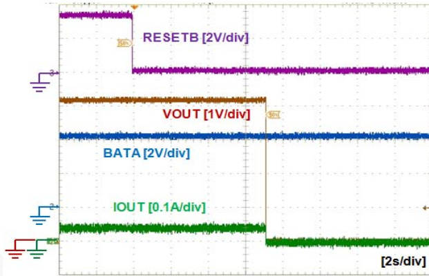
Figure 34. System Reset by RESETB: HIGH → LOW ( V_{BATA}=V_{BATB}=4.2V , C_{OUT}=100\mu F , R_L=100\Omega )
