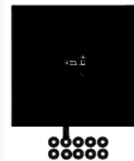
Figure 4. 1 Square Inch of 2-ounce copper
