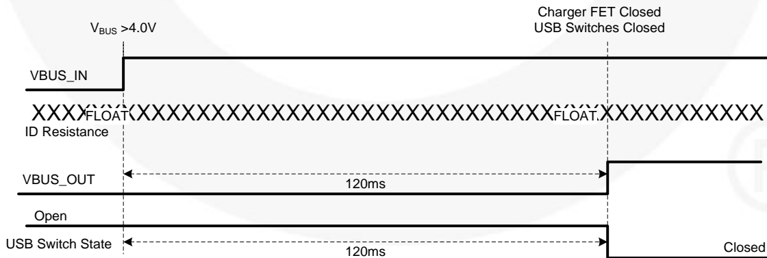
Figure 10. USB Standard Downstream Port Attach Timing (19)
