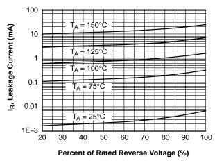
Figure 4. Typical Reverse Characteristics
