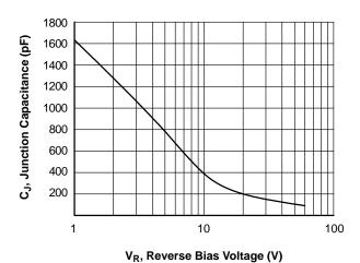
Figure 5. Typical Junction Capacitance
