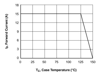
Figure 6. Forward Current Derating Curve
