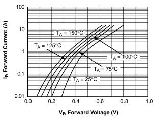
**Figure 3. Typical Forward Characteristics**
