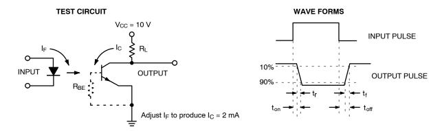
Figure 11. Switching Time Test Circuit and Waveform
