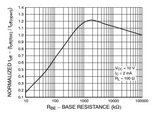
Figure 9. Normalized toff vs. RBE
