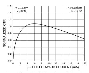
Figure 2. Normalized CTR vs. Forward Current
