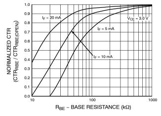
Figure 5. CTR vs. RBE (Saturated)
