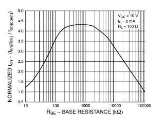
Figure 8. Normalized ton vs. RBE
