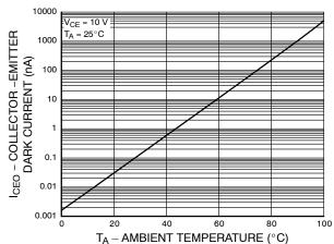
Figure 10. Dark Current vs. Ambient Temperature
