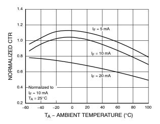
Figure 3. Normalized CTR vs. Ambient Temperature
