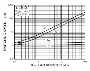
Figure 7. Switching Speed vs. Load Resistor
