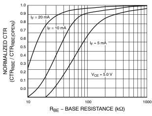
Figure 4. CTR vs. RBE (Unsaturated)
