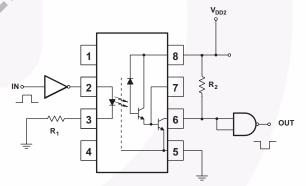
Fig. 3 Inverting Logic Interface
