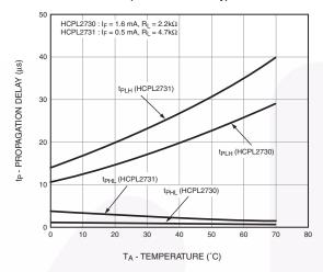
Fig. 23 Propagation Delay vs. Temperature (HCPL2730 / HCPL2731 Only)
