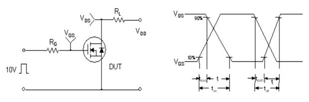
**Unclamped Inductive Switching Test Circuit & Waveforms**
