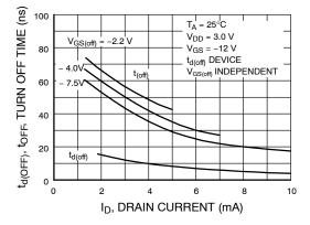
Figure 16. Switching Turn-Off Time vs. Drain Current
