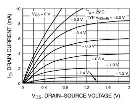
Figure 1. Common Drain–Source
