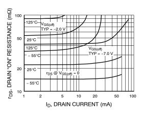
Figure 7. On Resistance vs. Drain Current
