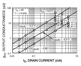
Figure 10. Output Conductance vs. Drain Current
