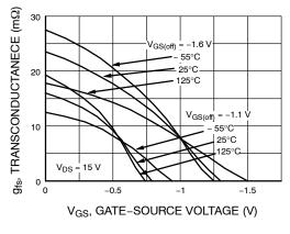
Figure 6. Transfer Characteristics
