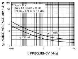
Figure 12. Noise Voltage vs. Frequency
