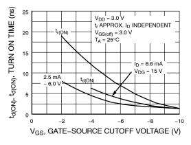
Figure 15. Switching Turn-On Time vs. Gate-Source Voltage
