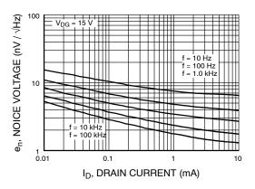
Figure 13. Noise Voltage vs. Current
