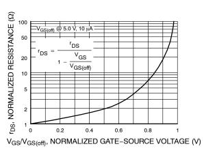
Figure 8. Normalized Drain Resistance vs. Bias Voltage
