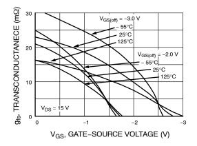
Figure 5. Transfer Characteristics
