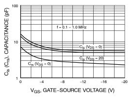
Figure 11. Capacitance vs. Voltage
