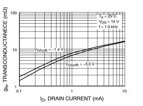
Figure 9. Transconductance vs. Drain Current
