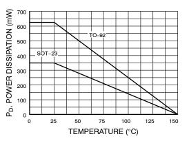
Figure 14. Power Dissipation vs. Ambient Temperature
