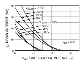
Figure 3. Transfer Characteristics
