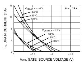
Figure 4. Transfer Characteristics
