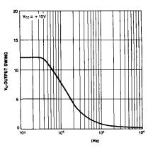
Figure 4. Large Signal Output Swing vs Frequency
