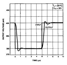
Figure 12. Voltage Follower Pulse Response (Small Signal)
