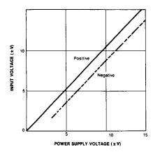
Figure 7. Input Voltage Range vs Supply Voltage
