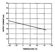
Figure 9. Output Current vs Temperature (Current Limiting)
