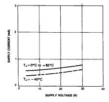
Figure 1. Supply Current vs Supply Voltage
