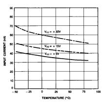
Figure 10. Input Current vs Temperature
