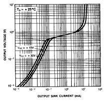
Figure 6. Output Characteristics vs Current Sinking
