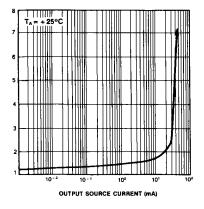
Figure 5. Output Characteristics vs Current Sourcing
